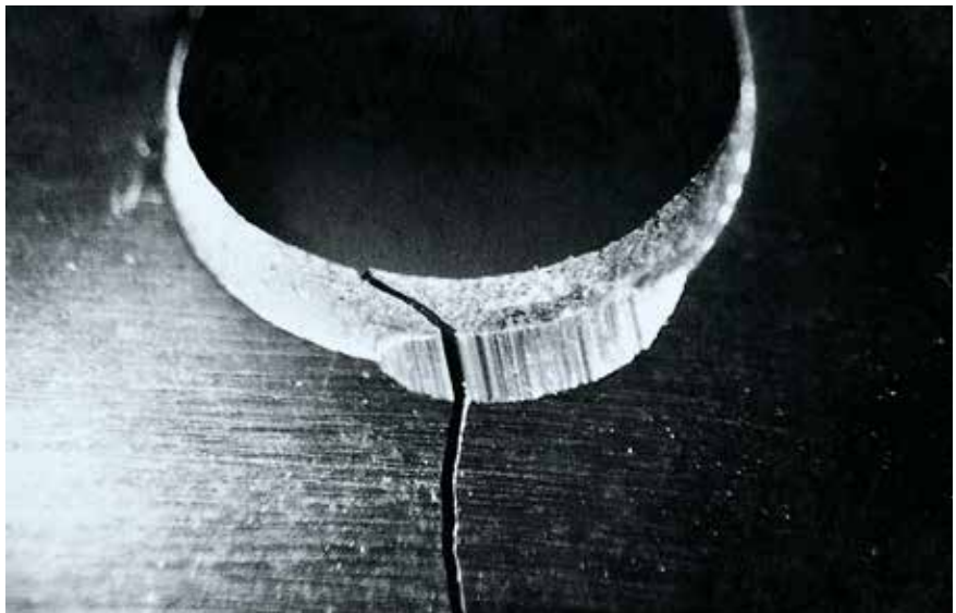
Fracture in the saw body.
